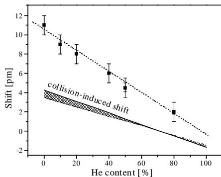
Fig.2 The measured shift (squares) and the collision-induced shift calculated from [3]
