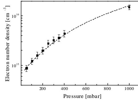
Fig.3 Extrapolation of the electron density results obtained in the pressure range 50 mbar – 400 mbar
